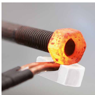
Releasing of rusted bolts
