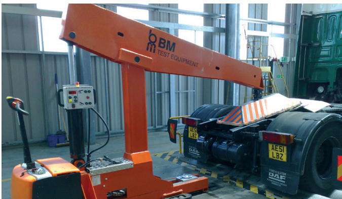
CLS applied to chassis from top-down
